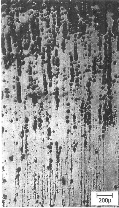
Fig.1 Microstructure of the longitudinal cross section of irradiated and annealed cylindrical wire Cu/0.085wt% B alloy specimen in as-polished condition [1].
