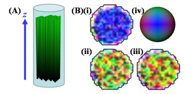
Figure 1: Diffusion tensor imaging results for the self-diffusion of water in a templated hydrogel after storage. (A) Schematic of the alignment in the hydrogel in a 5 mm Wilmad NMR tube. (B) Diffusion tensor images for an axial slice (voxel size:  $0.196 \text{ mm} \times 0.196 \text{ mm} \times 0.5 \text{ mm}$  (slice thickness), diffusion time: 70 ms). (B)(i), (ii) and (iii) show images for the first, second and third eigenvectors, and (iv) a directional representation.
