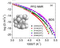
Fig. 1: Diffusion coefficients determined from broadband dielectric spectra by employing the Einstein-Smoluchowski equation (using  $\omega_c$  as the characteristic hopping rate) and independently measured by PFG NMR (open symbols). The lines denote fits by the Vogel-Fulcher-Tammann equation. Inset: One of the possible conformations of the [OMIM] cation.
