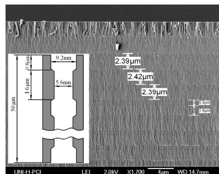
Fig. 1. SEM image of the cross section of one of the used PSi samples with a modulated structure revealing layers with different porosities (pore sizes). The inset shows the expected pore structure.
