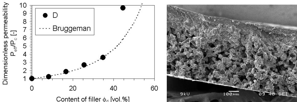
Fig. 1: The comparison of experimental  $P_{eff}/P_c$  vs.  $\phi_d$  plot for membrane made of PI(6FDA-ODA) with theoretical dependence simulated using the model by Bruggeman.
