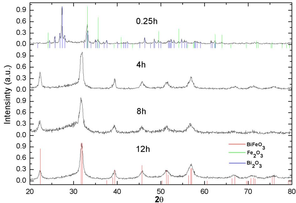
Fig. 1 X-ray diffraction of Fe<sub>2</sub>O<sub>3</sub>/Bi<sub>2</sub>O<sub>3</sub> milled for: 0.25 h, 4 h, 8 h and 12 h.
