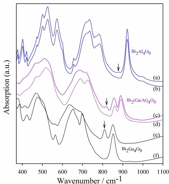
**Fig. 1** FTIR absorption spectra of samples with compositions  $\text{Bi}_2\text{Al}_4\text{O}_9$  (a, b),  $\text{Bi}_2(\text{Ga}_{0.6}\text{Al}_{0.4})_4\text{O}_9$  (c, d) and  $\text{Bi}_2\text{Ga}_4\text{O}_9$  (e, f) in air heated (96 h at 800 °C) before (a, c, e) and after (b, d, f) heating in  $^{18}\text{O}_2$  (16 h at 800 °C).
