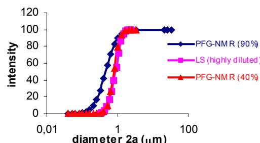
**Fig. 2** Droplet size distribution of an emulsion of paraffin oil obtained by PFG-NMR and light scattering (LS).
