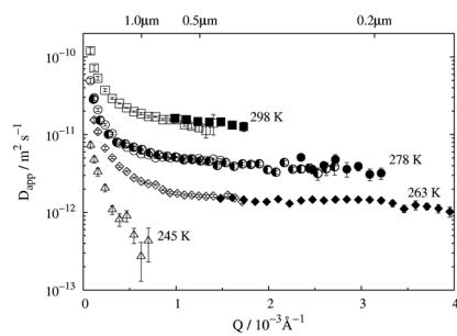
Fig. 2  $Q$ -dependence of the apparent diffusion coefficient  $D_{\text{app}}$  of  $\text{H}_2\text{O}$  in polycrystalline NaA-zeolites as obtained by fits of eq. 1 to experimental echo decay curves in a magnetic field gradient (open symbols: 58 T/m; half-filled: 135 T/m, filled: 185 T/m).
