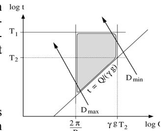
Fig. 1 Schematic representation of the working range (shaded area) of FG-NMR in confined geometries.
