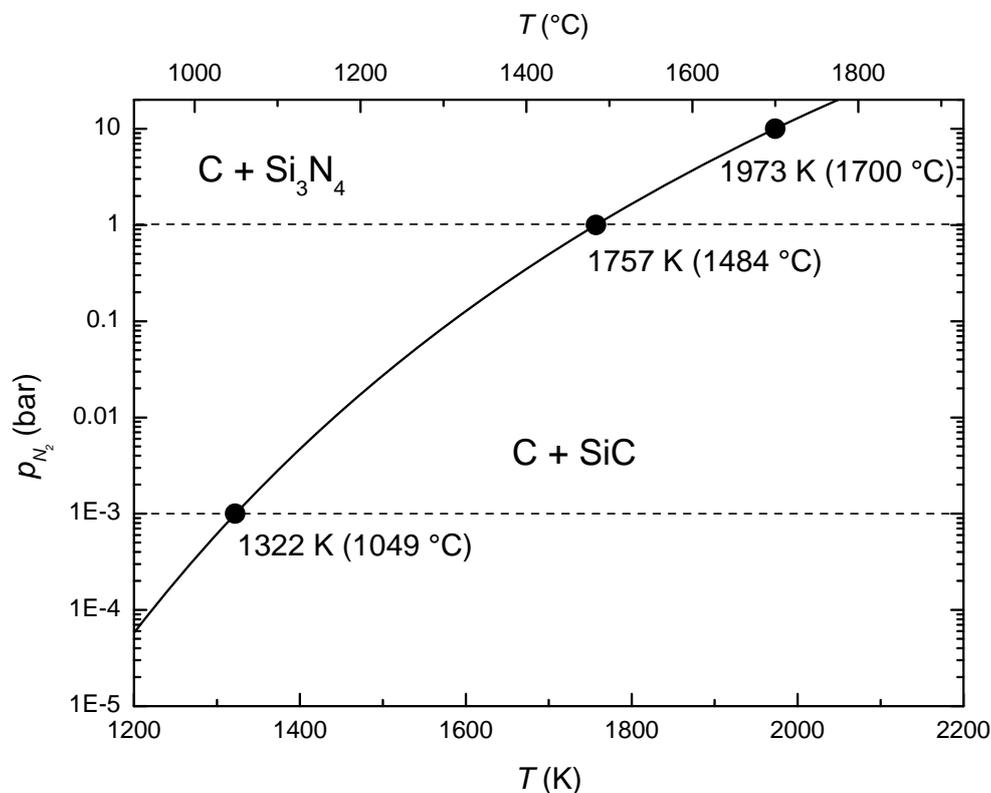
**Fig. 1:** Phase diagram of the VT50C ceramics after ref. [5]. Indicated are the nitrogen partial pressures used in this work as dashed lines.
