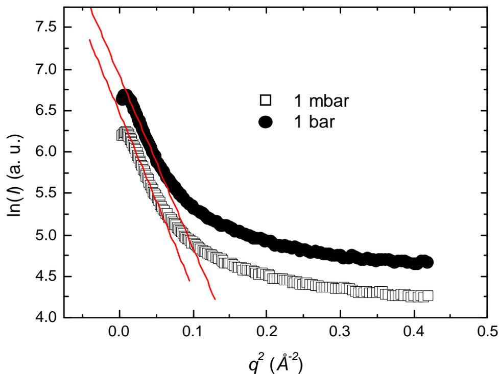
**Fig. 2:** Guinier representation of the SAXS intensity  $I$  for VT50C samples annealed at 1500 °C for 70 minutes at a nitrogen partial pressure of 1 bar and 1 mbar, respectively. The upper spectrum was shifted for clarity.
