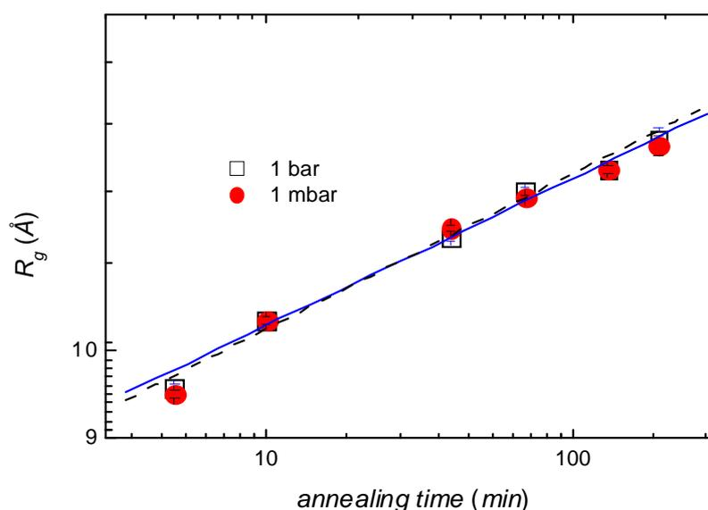
**Fig. 3:** Double logarithmic plot of  $R_g$  versus annealing time  $t$  for the samples annealed at a nitrogen partial pressure of 1 bar and 1 mbar, respectively.
