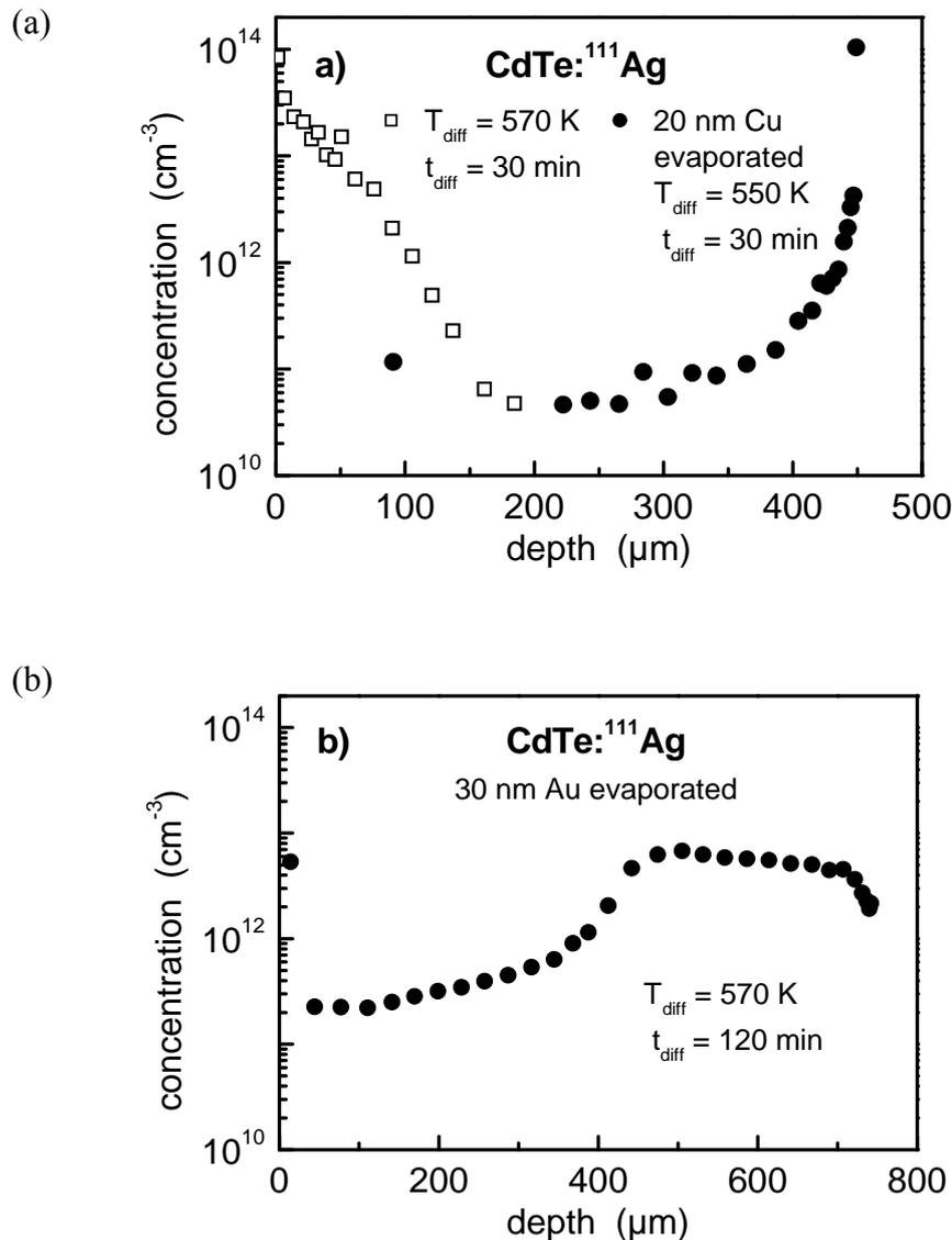
**Fig. 2:**  $^{111}\text{Ag}$  profiles in CdTe measured after implantation of  $^{111}\text{Ag}$  and evaporation of (a) a Cu layer (filled circles) and (b) a Au layer onto the implanted surface. In panel (a) (open squares) additionally the Ag profile obtained without evaporated metal layer is shown. Note the different thicknesses of the crystals in (a) and (b)
