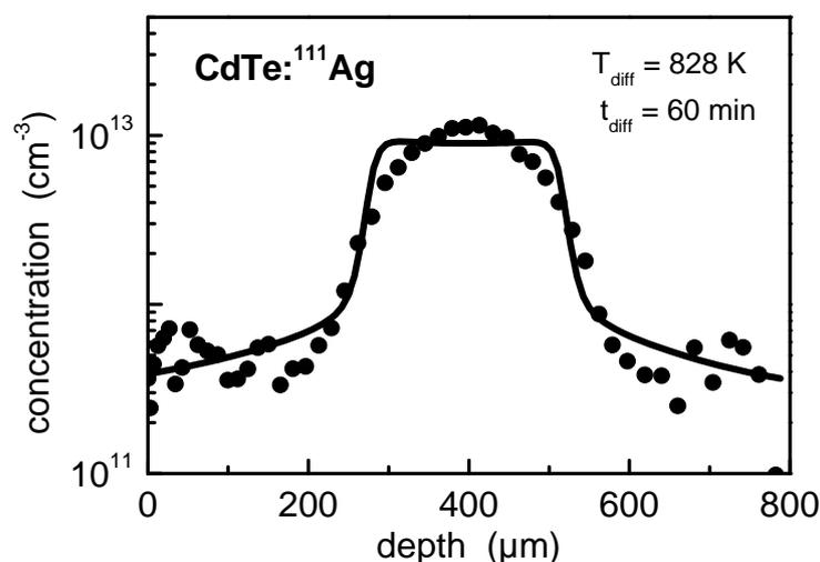
**Fig. 1:**  $^{111}\text{Ag}$  profile in CdTe obtained after diffusion at 828 K for 60 min under Cd pressure. The solid line corresponds to a simulation according to the model described in sec. 4.
