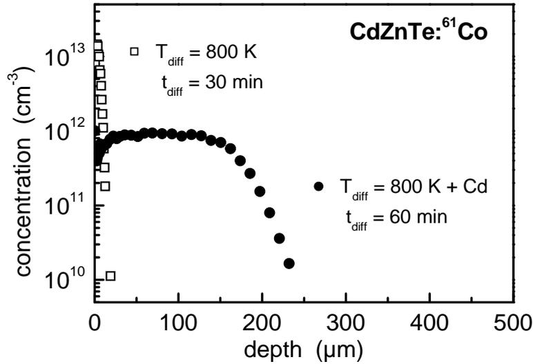
**Fig. 3:**  $^{61}\text{Co}$  profiles measured after implantation and subsequent annealing under Ar atmosphere (open squares) and under Cd pressure (filled circles).
