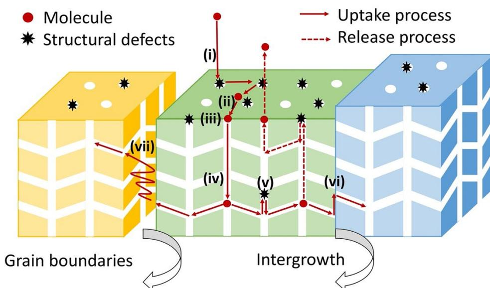
**Fig. 1.** Illustration of the transport process from the bulk phase into the interior of nanoporous materials. From Xu et al. [5]
