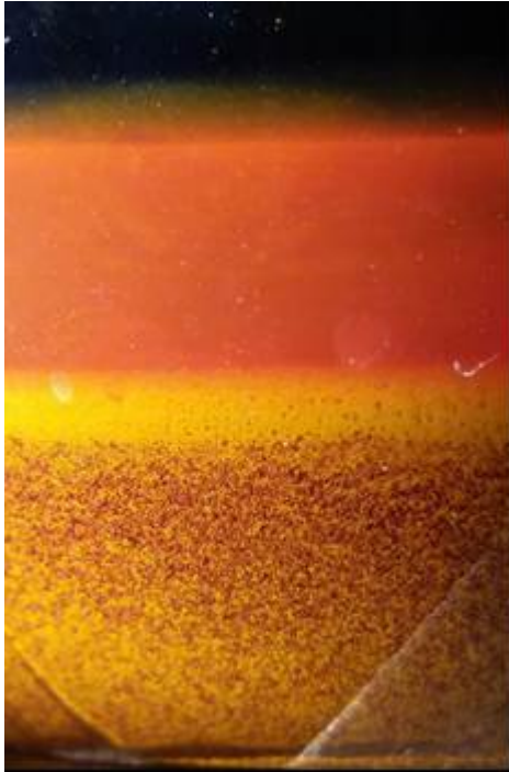
Fig. 2: Typical picture after 3 days of stirring and subsequent sedimentation. Upper (black) layer - NaCl+V 2 O 5 - solution in water, red layer - V 2 O 5 -nano crystals, yellow layer – “semi-product”, bottom layer – untransformed V 2 O 5 powder
